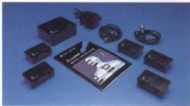
networks are joined together using Bridges. These provide high speed automatic connection between separate Econet networks. One of the advantages of joining networks together in this way is that if one section of the network fails, the rest of the Econet system is not affected.
